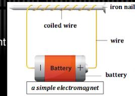
Another way to look at this is that a moving electrical current creates a magnetic field, and a moving magnetic field creates an electrical current. This tightly **coiled wire** that produces a magnetic field when electricity passes through the wire is called an electromagnet.
