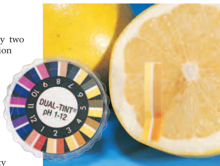
Figure 14 The paper strip contains several indicators. The pH of a solution is determined by comparing the color of the strip to the scale provided.
