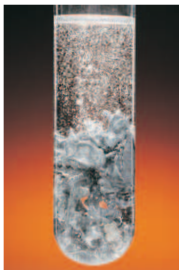
Figure 7 Bubbles of hydrogen gas are produced when zinc metal reacts with hydrochloric acid.
