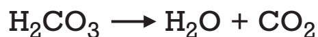
Figure 16 A model for the decomposition reaction of carbonic acid to form water and carbon dioxide is shown below.
