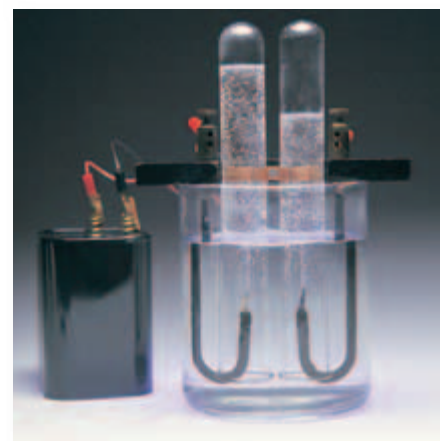
Figure 15 Water can be decomposed into the elements hydrogen and oxygen through electrolysis.
