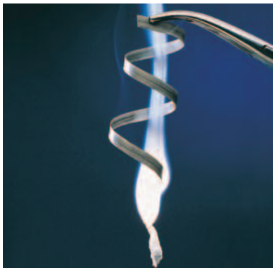
Figure 13 The synthesis reaction that occurs when magnesium reacts with oxygen in the air forms the compound magnesium oxide.
