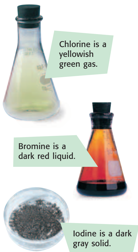
Figure 12 Physical properties of some halogens at room temperature are shown here.
