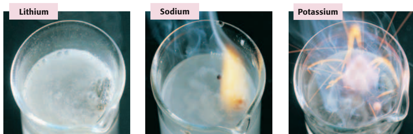
Figure 5 As alkali metals react with water, they form hydrogen gas.
