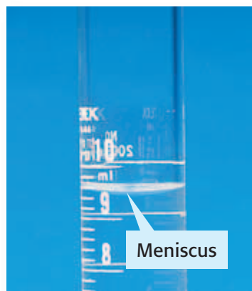
Figure 3 To measure volume correctly, read the scale at the lowest part of the meniscus (as indicated) at eye level.
